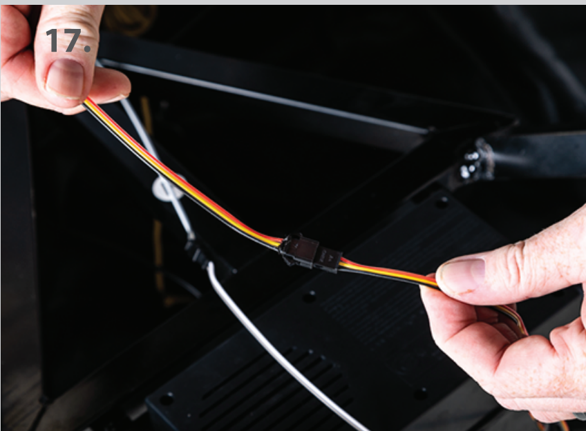
17. Connect red wire to red wire of control box.
